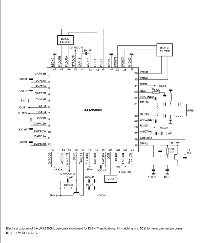
Fig.3 Demonstration board diagram.
